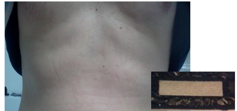
Embroidered electrodes after long term wear test (10 days)
